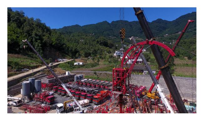
The Apollo Turbine Fracturing Pumper Working for Shale Gas Production
